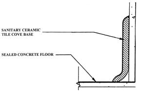
TYPICAL COVE BASE DETAIL ON CONCRETE FLOOR
